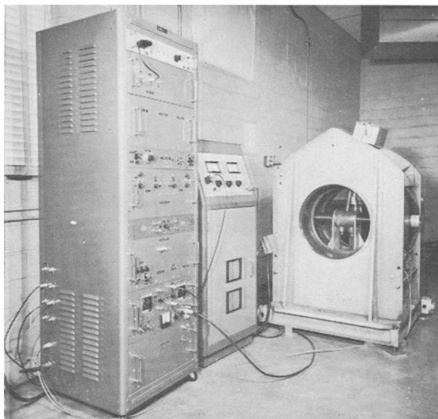
FIG. 8. NMR equipment developed at Southwest Research Institute to measure the amount of hydrogen in a 3 in. flowing process stream.
